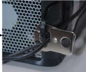
Steel cable trap captures and secures Dell CPU, internal components, mouse and keyboard cables.
