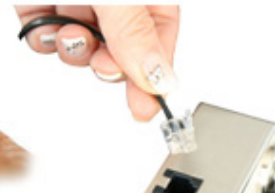
The sensor loop plugs into the alarm module. Cutting or unplugging triggers the alarm
