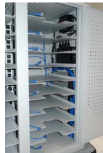
Fan, electronic switching timer, 48 port network switch and Ethernet cables all pre-installed
